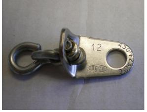
ML (Max Load) fusible metallic link dated 2012; temperature rated 232°C/450°F
